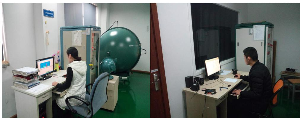
**Figure 5: The LEDs are carefully tested for its spectral power distributions and spatial distribution using calibrated 1.5m integrating sphere and GO2000.**
